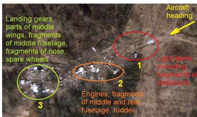
**Fig. 1.** The Tu-154M PLF 101 wreckage trail plot grouped by location of parts of the aircraft: (1) light items including fragments of stabilizers; (2) engines, fragments of middle and rear fuselage, rudder; (3) landing gears, parts of middle wings, fragments of middle fuselage, fragments of nose, spare wheels.
