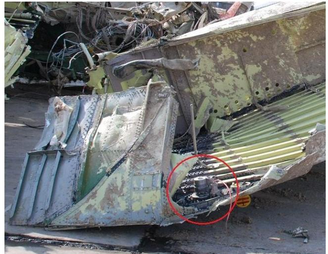
Fig. 18. Fuel booster pump ЭЦН-325 of the wing fuel tank in the left centerwing. Photograph taken at the place of storage of the wreckage. Source: [www.fakty.molensk.gov.pl](http://www.fakty.molensk.gov.pl) [7].
