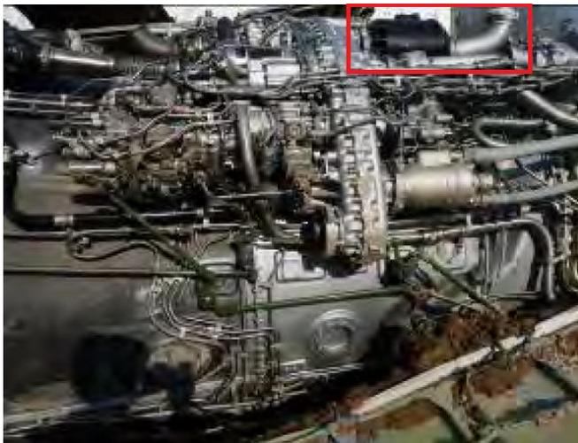
Fig. 4. Generator ГТ40ПЧ6 on the engine No 1 (left). The engine cover (cowl) has been removed. Photo taken between 11 and 13 April 2010 on the crash site. Source: Annexure No 4.10.22 to KBWLLP Report [6].
