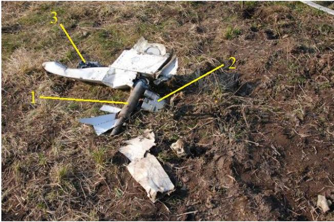
Fig. 11. Screw actuator for left wing flaps (1), electromagnetic brake ТЭМ-4 (2) and reducer (3). Photo taken by IAC (MAK) [8] Source: [www.faktysmolensk.gov.pl](http://www.faktysmolensk.gov.pl)
