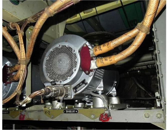
Fig. 5. Rectifier BY-6Б 208 V 400 Hz/27 V DC on the Tu-154 aircraft. Source: <http://commons.wikimedia.org/wiki/File:VU-6B-rectifying-device-on-Tu-154.jpg>
