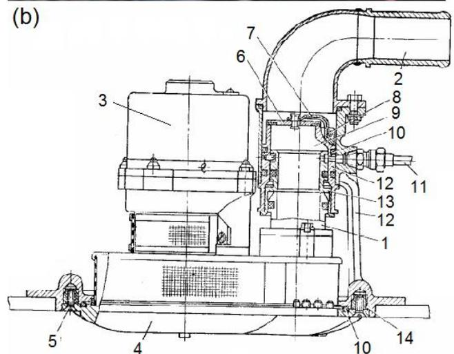
Fig. 19. Identification of the fuel booster pump ЭЦН-325: (a) magnified circled area of Fig. 18; (b) outline of the fuel booster pump ЭЦН-325 [3]: 1 - tubes, 2 - induction motor driven pump, 3 - cover, 4 - screw, 5 - disk cover, 6 - lever, 7 - spring, 8 - non-return valve, 9 - rubber ring, 10 - pipeline, 11 - body, 12 - base, 13 - fittings.
