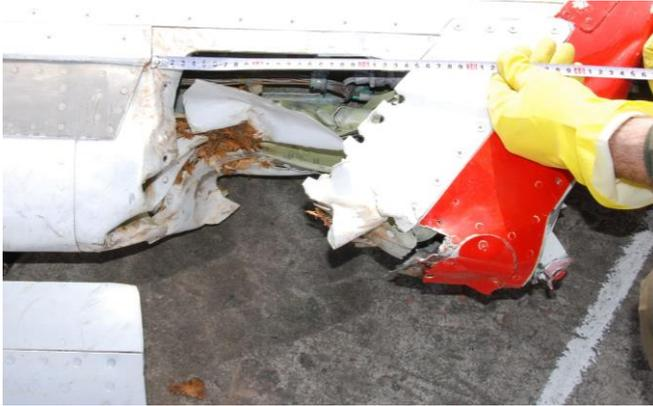
**Fig. 20.** A bundle of electric wires located before front spar of the detached portion of left wing. The front skin has been probably damaged when the severed part of wing hit the bushes at the crash site, while dropping. Note that slat covering the front skin has not been damaged Source: [www.faktysmolensk.gov.pl](http://www.faktysmolensk.gov.pl) [14 7].
