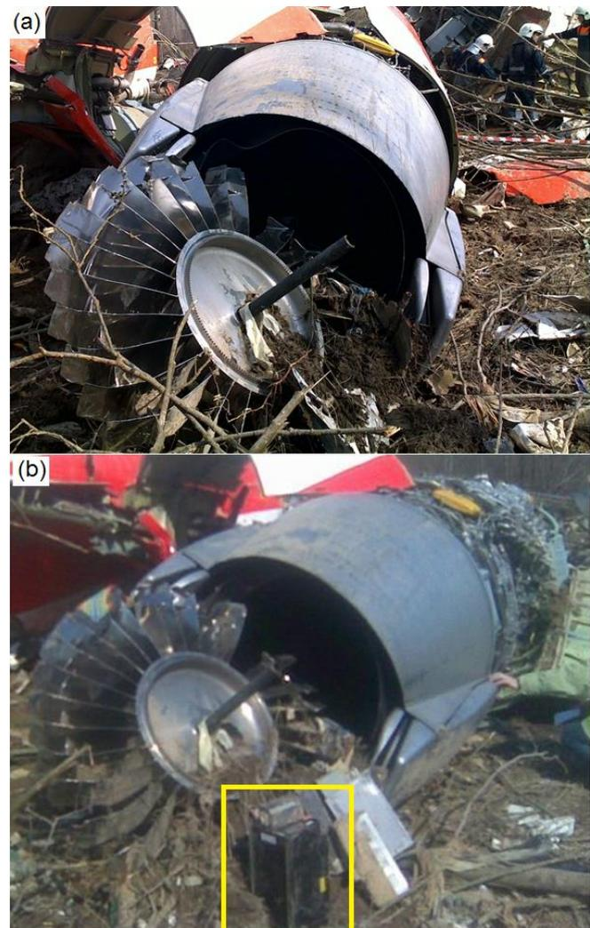
Fig. 15. Low pressure compressor (LPC) of the left engine No 1 at the crash site. (a) the blades were spinning before touching the ground because their tip portion is covered with soil (b) the object in rectangular frame beside the LPC is probably the battery 20HKБН-25-Y3. Source: Fig. 15a [www.faktysmolensk.gov.pl](http://www.faktysmolensk.gov.pl) , Fig. 15b unknown source.
