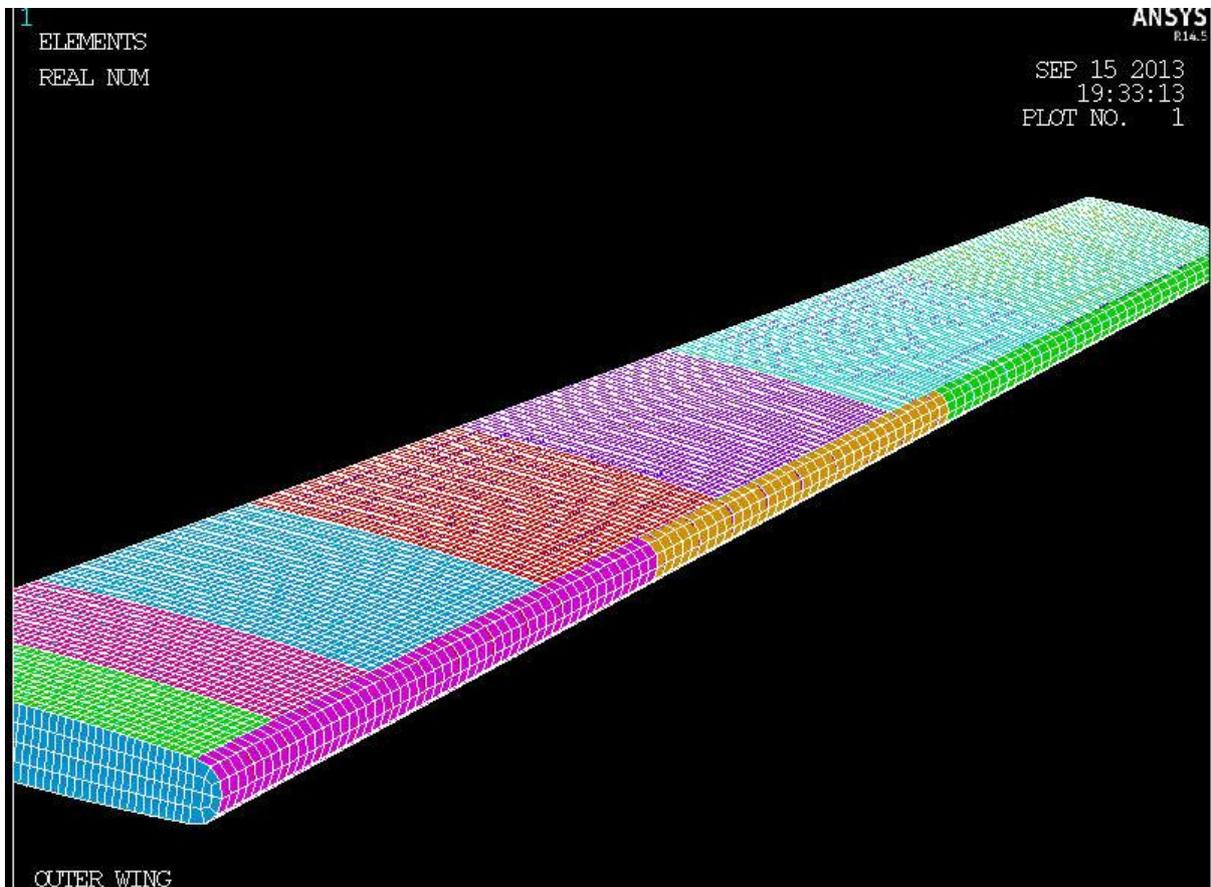
Fig. 2. Over-all view showing the top skin divided into seven chordwise segments as well as the nose skin divided into three segments.
