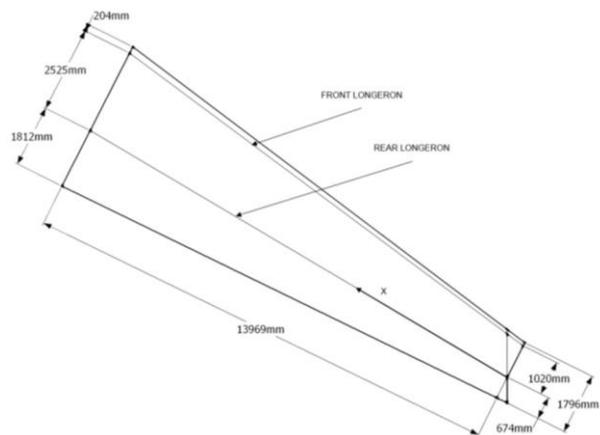
**Fig. 1. Simplified outer wing, outline in plan view. The wing tip was slightly altered to make it parallel to the root section.**
