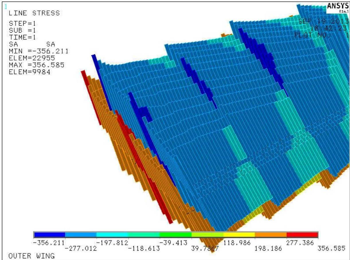
Fig. 5. Axial stress in stringers plotted at right angle.
