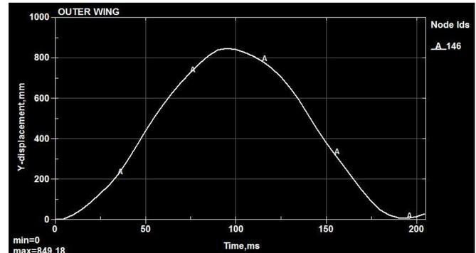
Fig. 7. Vertical displacement of the wing tip following the step loading of pressure.
