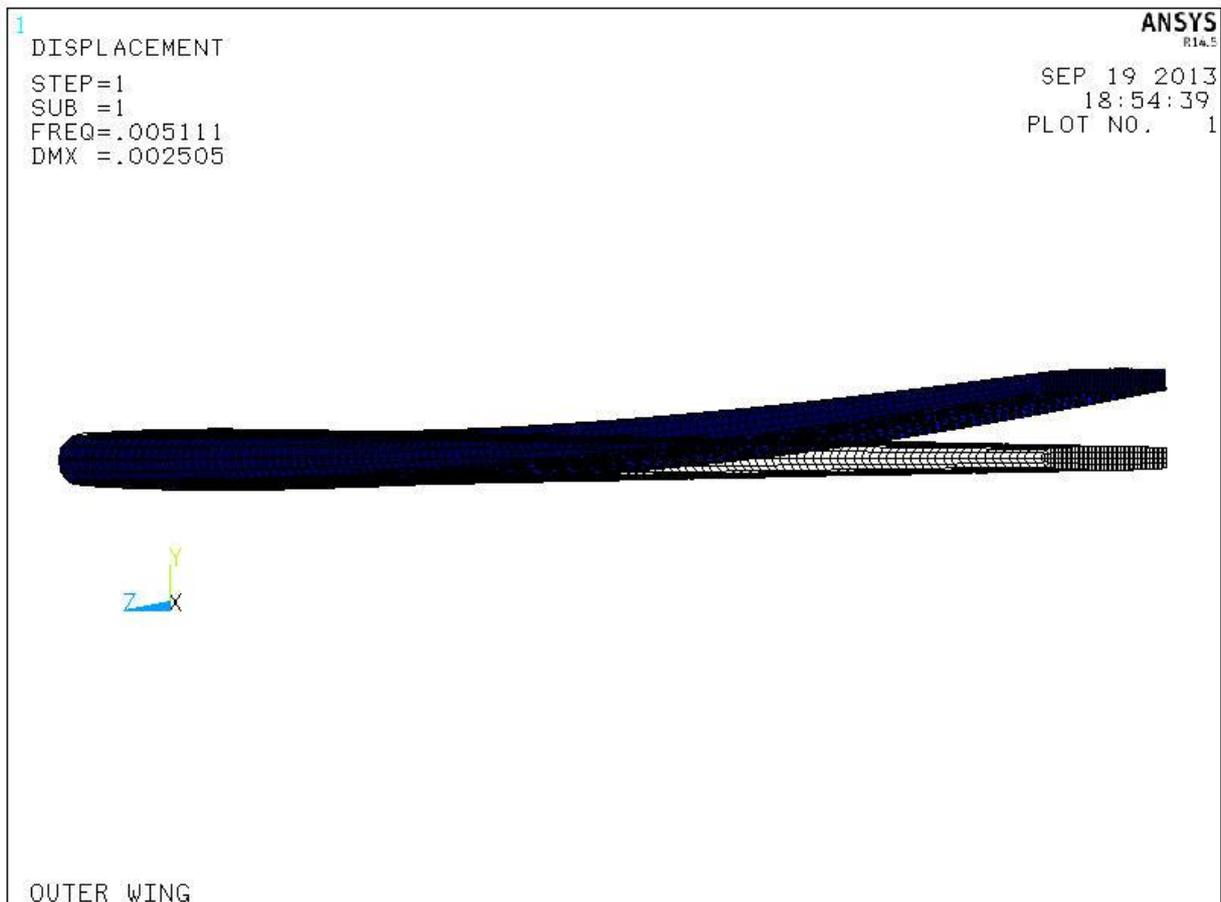
Fig. 6. The first natural mode of vibration, bending, at 5,11 Hz.
