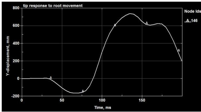
Fig. 9. Tip displacement caused by the root section movement.
