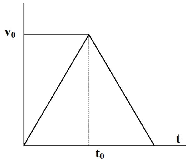
Fig. 8. Applied vertical displacement at the root section.
