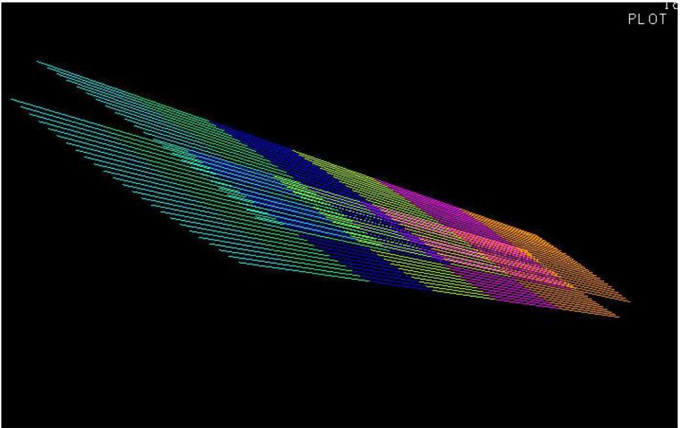
Fig. 3. Six segments with different properties of stringers are marked. The left, right and center stringers serve as longeron caps.
