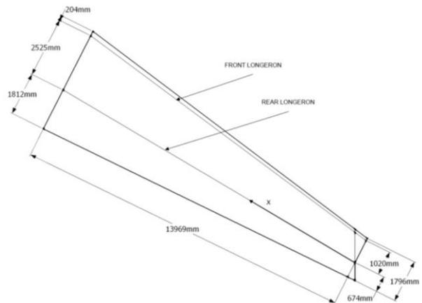
**Fig. 1. Simplified outer wing, outline in plan view. The wing tip was slightly altered to make it parallel to the root section.**
